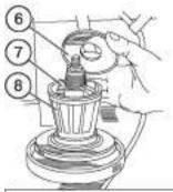
**Note:** After diesel stop, for 30-60 seconds noise of rotating rotor should be audible. It means that filter functions properly.
