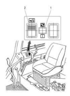
**Note:** The electric circuit of FDA drive control is provided with braking relay, ensuring automatic FDA drive switching on upon pressing interlocked wheel brake pedals. It is installed only on the models where FDA drive is aligned with DI.
