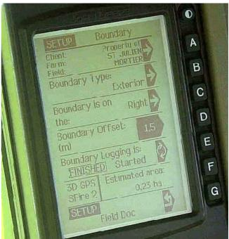
GreenStar Field Doc offers a simple way to record information on operations including tillage, seeding, spraying, fertilising and in applying manual or automatically variable input rates required for modern farm documentation practices. In addition, customers can also draw upon a simple and highly accurate boundary measurement tool incorporated into the Field Doc system.
