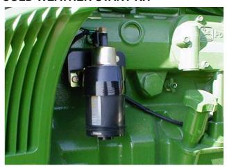
The introduction of a pilot injection system on the 8020 Series tractors reduces the need for use of the ether starting aid. Should customers frequently start tractors at or below -6 degrees Celsius however, a Cold Weather Start kit is recommended and available for field installation.
