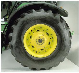
Customers utilising the *Substitutable Rear Shipping Wheels* option can source rims to mount on the Heavy Duty Cast hub and centres supplied with the tractor.
