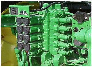
The attachment kit includes a fourth SCV, SCV control assembly, potentiometer, wiring harness, couple with release lever, dust cover and installation hardware & instructions.
