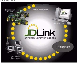
The innovative GreenStar JDLink system from AMS allows customers to optimise the true performance capabilities of their 8020 by collecting machine data for management purposes. Using mobile phone technology, JDLink continuously transmits signals from the tractor's CAN Bus system to a central John Deere server where the information can then be made available to users via a JDLink website or through email, fax or SMS messaging.
