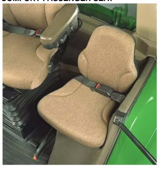
Comfort Passenger Seat provides a comfortable, and convenient location to sit while instructing new or inexperienced operator.
