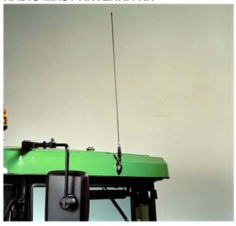
External radio mast antenna kit can be supplied to improve the radio reception on tractors equipped with an internal roof antenna. The external antenna is mounted with a three-position rosette and allows 90° forward / rear rotation to avoid damage from contact.
