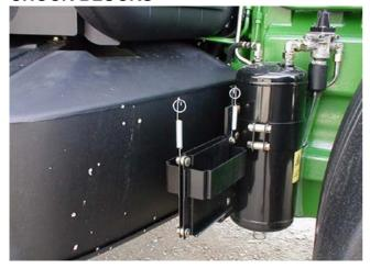
Chock blocks are advised for use as an additional safety measure when parking tractor / trailer combinations and to fulfil statutory regulations where required. Additional Block Holder bracket can be assembled when not previously supplied ex-factory (see Parts Catalogue).
