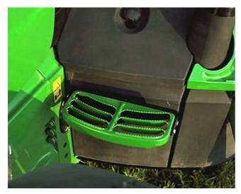
The left hand step provides convenient access to the front window for cleaning and also for GreenStar StarFire Receiver mounting and dismounting:
