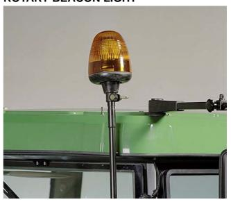
Rotary beacon lights are available to meet requirements in commercial or governmental applications. The rotating, high-intensity light mounts on the front left corner of the cab roof in the up position when in use and can be lowered when not required to prevent damage. On / Off switch for the beacon light is located within easy reach of the operator.
