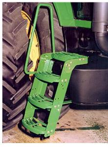
The right-hand step kit includes full-sized steps and handrail as well as an individual step on the left side for improved cab access.
