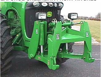
Approved front hitches are available for both Independent Link Suspension and regular 4WD front axle tractors in two configurations: **Standard** and **Heavy Duty**.
