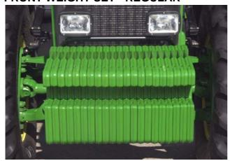
This attachment kit includes 20 Quick Tatch weights, each weighing 50 kg. There are 10 left front side weights and 10 right front side weights totalling 1000 kg.
