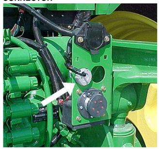
The 9-pin implement feedback connector required for TouchSet depth control of implements is available as a field-installed attachment. The connector and wiring harness enables a position input to be provided to the tractor's Selective Control Valve (SCV) control unit, enabling TouchSet depth control functionality. The feature allows the operator to adjust height and depth of remote lift cylinders by using the TouchSet controls in the cab.
